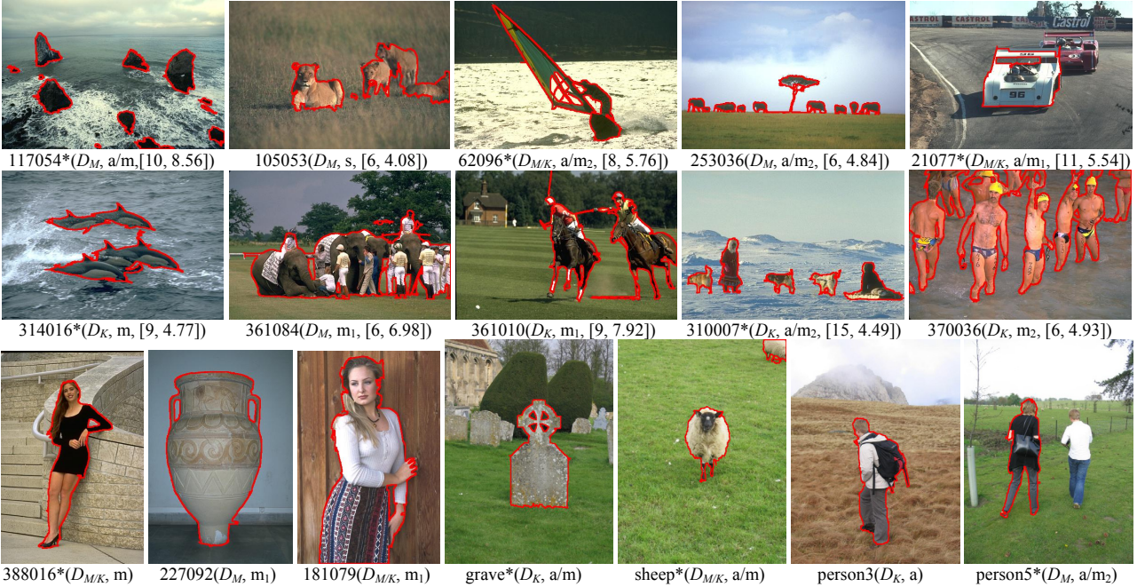
Figure 9. Example user-selected segmentations (*: coincide with auto-selection; s: voted by s-cut; a: voted by a-cut; m: voted by m-cut). The auto-selections (in supplemental materials) often coincide with the user-selections and are in general slightly worse in other cases.
